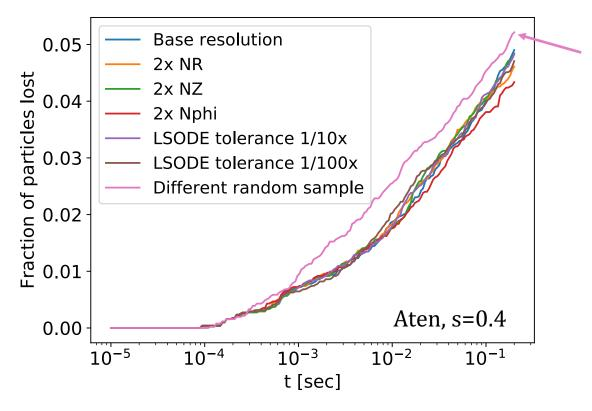
Same sampling algorithm & distribution, just a different initial seed, so the initial particle positions & velocities are different.
